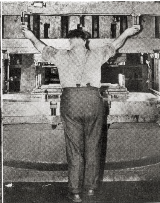
This Westinghouse worker can't injure his fingers. To bring down the press's "jaw" he must push two high-up control buttons.
